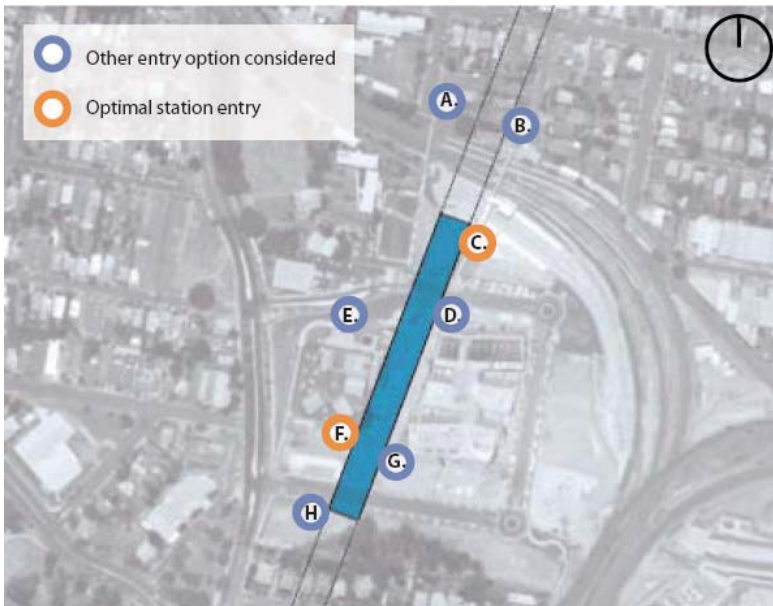
Figure 3-14 Boggo Road Station entrance location options
